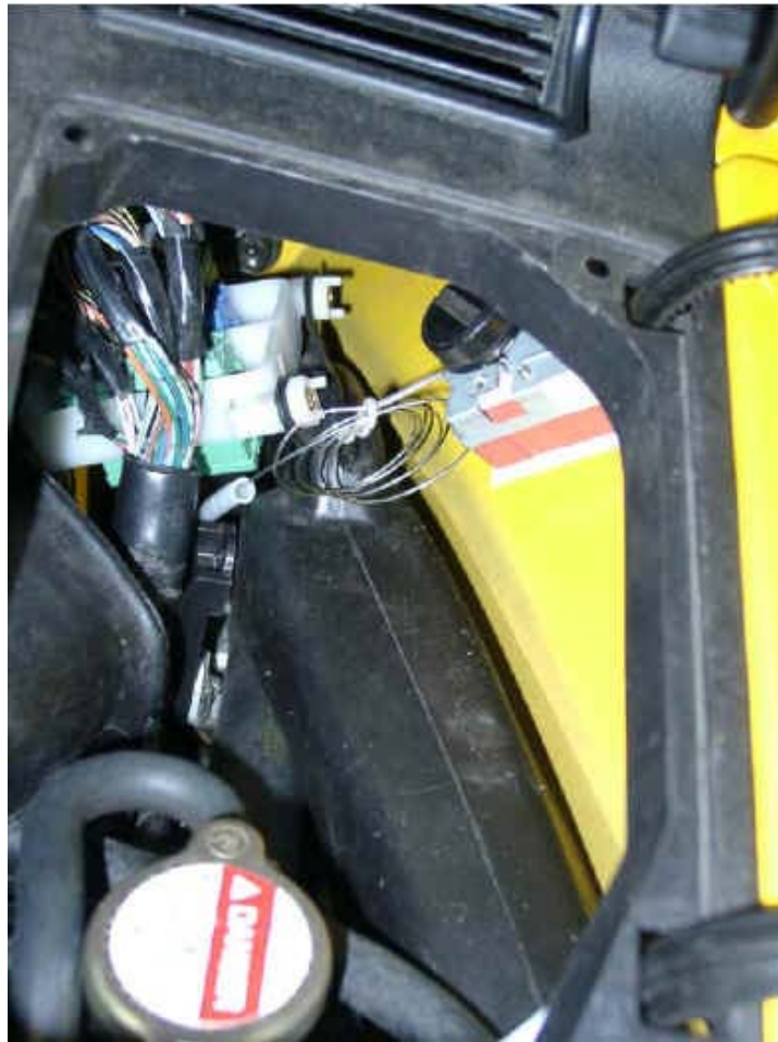
Thermostatic Switch Placed Inside Right Fairing Pocket
