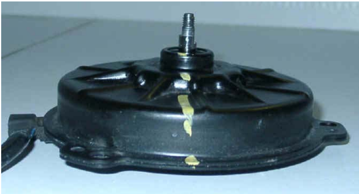
One Side of Shaft Cut
