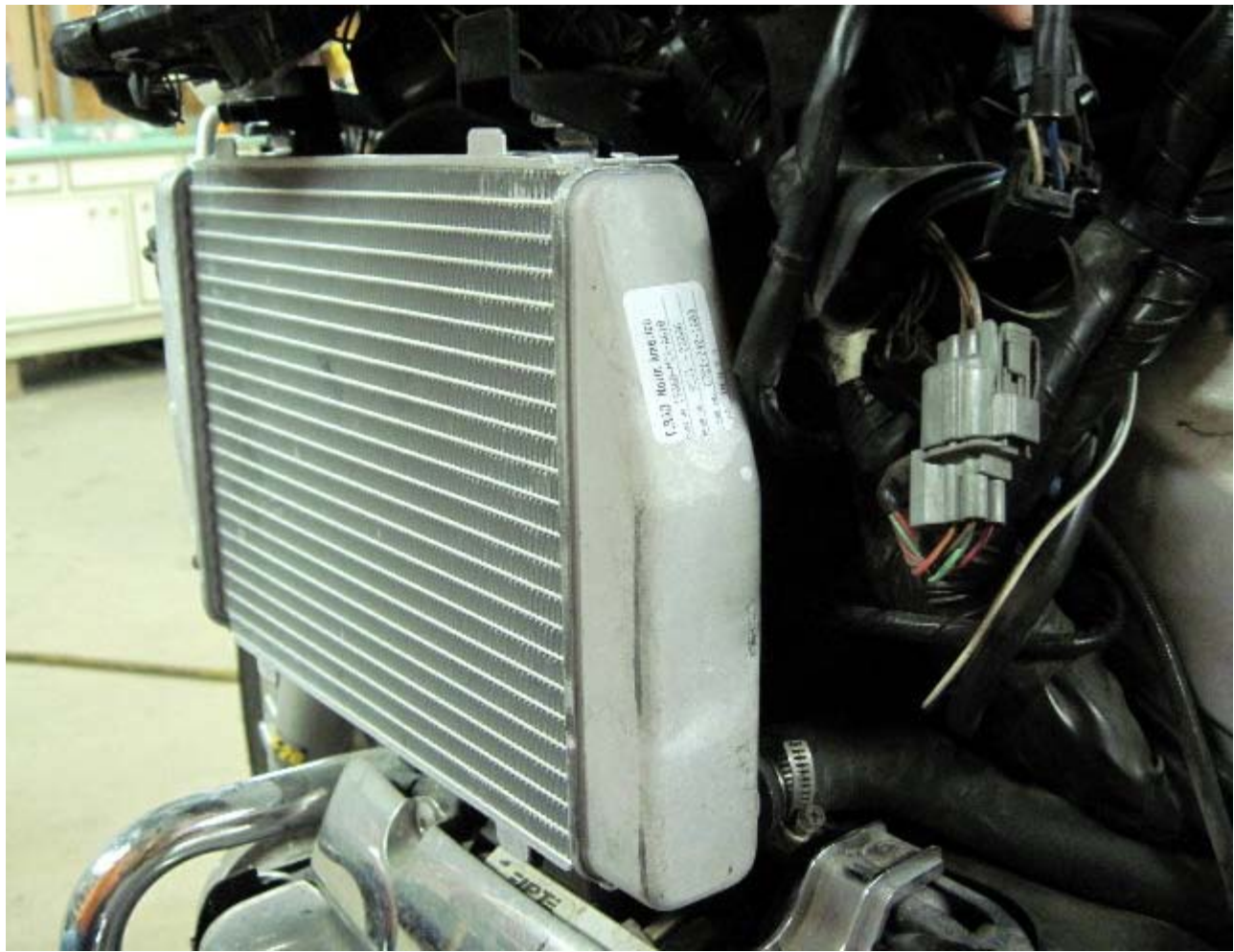
The left radiator installed.
