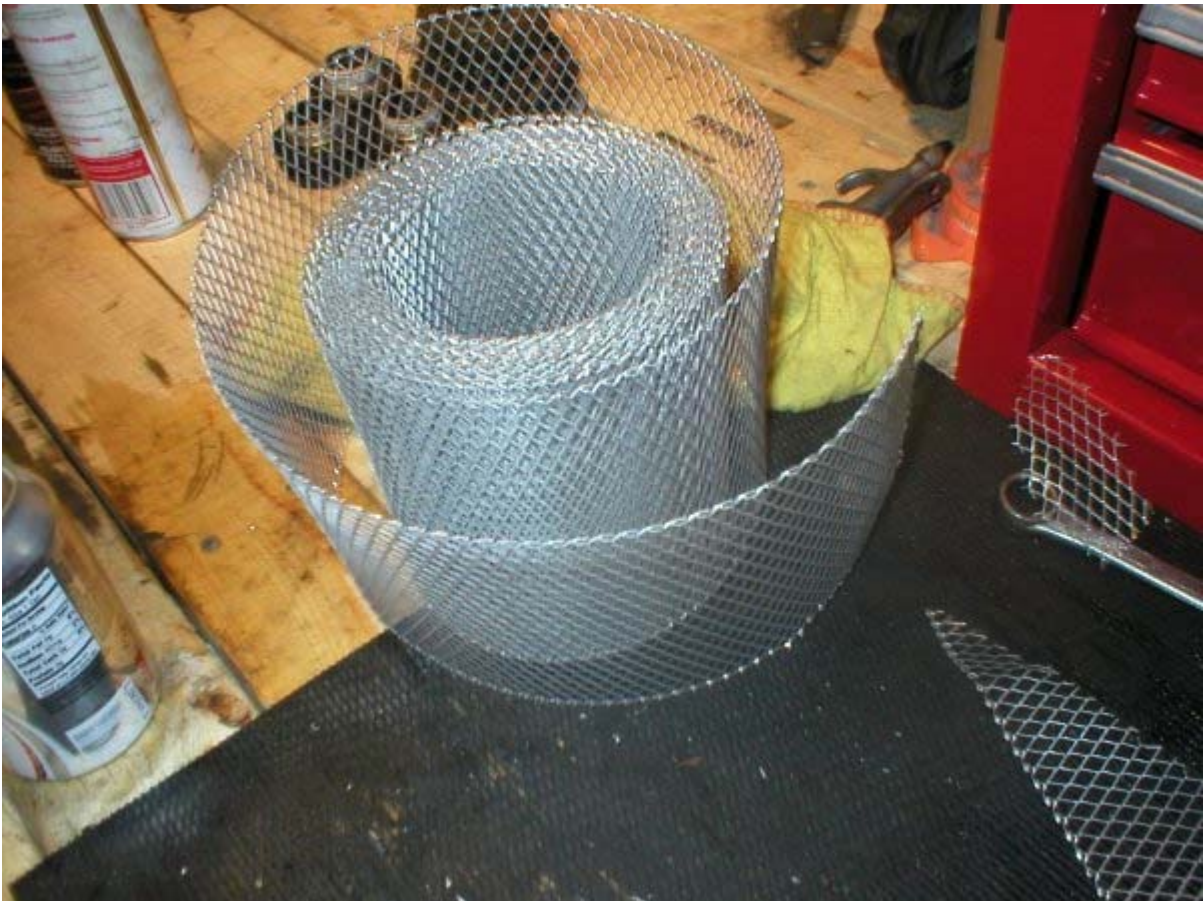
Hardware store roofing gutter screen is used to cover radiator intake area to keep dragon flies out along with debris and larger objects. This screen was only a few dollars and easy to shape as
