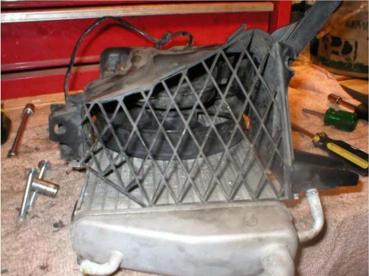
Normal configuration - fan clears radiator by approx 1/8"
