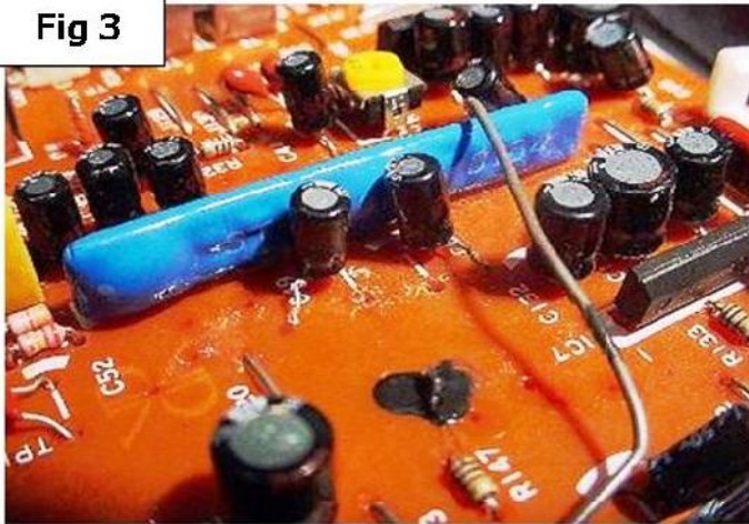
The positive legs are shown here de-soldered, pulled through to front of PCB and bent at an angle ready to accept the new wiring.
