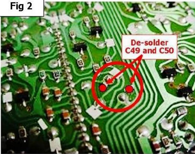
Turn PCB over, locate and de-solder capacitors C49 & C50. Shown in red circle.
